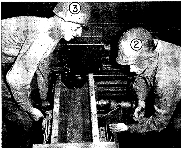
Figure 8. Nos. 2 and 3 removing traveling lock bracket.
